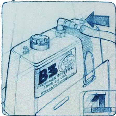
CONNECT SUPPLIED HOSE TO B3 UNIT. CUT TO LENGTH AND ATTACH
