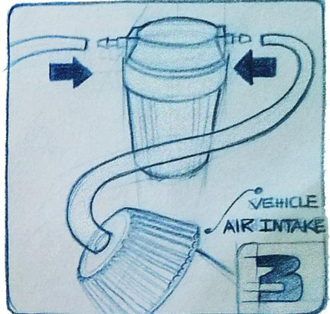
THE TOP OF THE BUBBLER, TO THE AIR DRYER. THEN A FINAL ONE FROM THERE TO THE AIR INTAKE.
