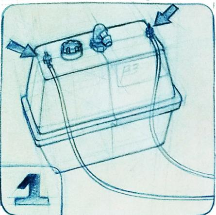
CONNECT CELL  $\ominus$  & CELL  $\oplus$  WIRES TO THE HYDROGEN CELL FROM THE SUPPLIED PWM UNIT.
