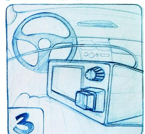
THE FUSE BOX. RUN THE DISPLAY WIRE INTO THE VEHICLE INTERIOR & MOUNT THE DISPLAY CASE
