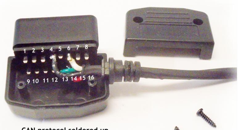
CAN protocol soldered up. Pin # 4 is (-) black. Pin #6 is white Pin #14 is green, Pin#16 is red (+).
