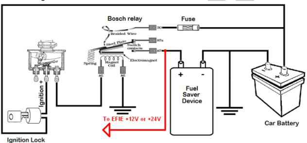
The reason which is necessary to connect +12 or +24 Volt of DEFIE to the +12 or +24 Volt of the fuel saver device is very simple: when you turn ON fuel saver device then simultaneously you turn ON DEFIE and when you turn OFF the fuel saver device then simultaneously you turn OFF the DEFIE. The DEFIE works only when the fuel saver device works. In any case you can use an ignition switched power source +12 or +24 Volt to the DEFIE. The DEFIE will shut OFF when you shut OFF ignition key.
