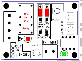
The best place for the installation of the DEFIE is a place where the DEFIE will be warm, dry and accessible to adjustment. As a last resort, the DEFIE can be placed under the hood, but you should take care of water resistance and humidity resistance. I recommend that is better to be installed under a dash. The DEFIE can be attached in the chosen place with Velcro. Due to this, it is necessary for you to pick up a suitable plastic box and attach the DEFIE inside with the Velcro.
