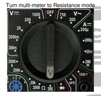
Test the resistance between ground wire, which you have found and battery negative terminal. If it is < 10 ohm you can use it.
