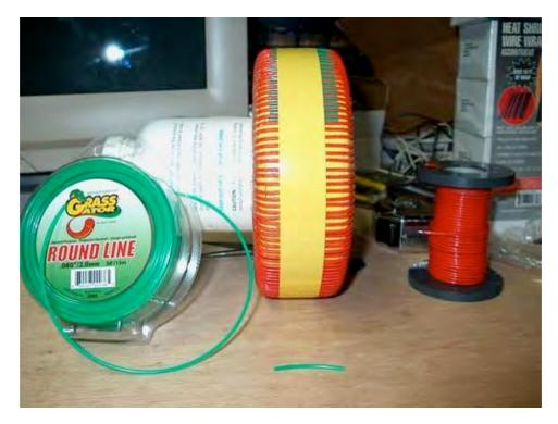
As you can see here, Bob uses short lengths of plastic strimmer cable as spacers for the outside of the toroid, though the picture above has been taken to show what a partially prepared secondary winding looks like when its windings are being moved into very accurate positions. The weed wacker spacers help you get accurate
