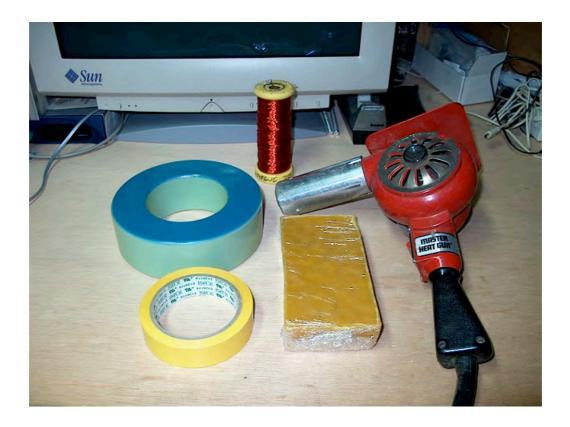
Of paramount importance with the toroid is that unlike traditional transformer design, the secondary is wound first, and the windings must be evenly spaced where they fan out from the center of the core. This means even though they are tightly packed right up against one another at the center hole, they must not be wound so that they bunch up and gap open around the periphery. Mistakes here will cause field errors that will lower the overall efficiency.
