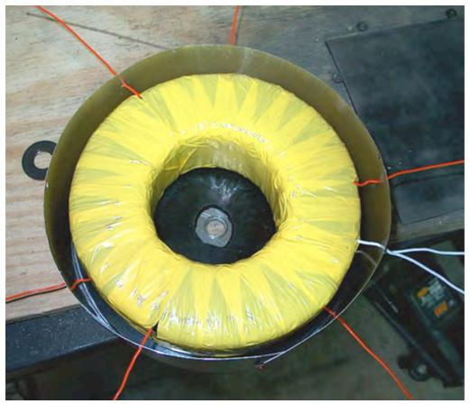
Please note the wires coming straight out, you will add posts on the cage itself, or place in another alum. box a rubber matt is on the bottom. Notice the wires coming off the top and bottom of the core, this is also important.
