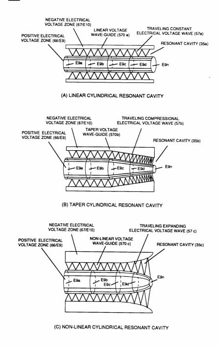
FIGURE 7-12: RESONANT CAVITY ELECTRICAL VOLTAGE WAVE
