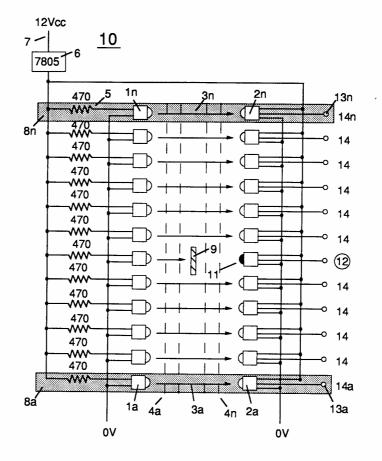
FIGURE 3-9: LED PICKUP CIRCUIT
