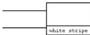
Figure 2 Negative lead of capacitor C4, white stripe to negative square hole. .
