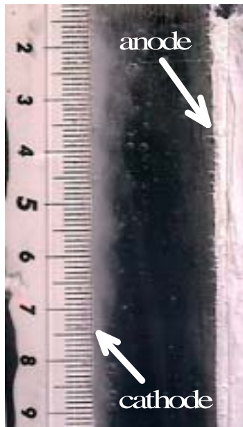
Fig.3 Two phase flow pattern between electrodes ( \Phi=1.0\text{A}/\text{cm}^2 , T=40^\circ\text{C} , C=40\% )
