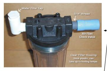
he black 3/4" fitting goes on the end of the check value, his allows a 1/2" OD black rubber outgas hose or 1/2" OD lear polyurethane tubing to fit inside the back fitting. I do not glue the hose in as a blow off safety feature in case of
