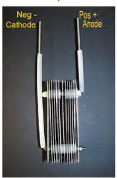
As you assemble the 13 plate set, keep in mind that you want to keep an even 1/8" spacing between the plates, as possible If it gets a little wider to 1/4" that is OK. The wide 1/8" nylon washers work well at keeping this 1/8" space, towards the center plate and end plates it usually goes a bit wider to 3/16" to 1/4" that is OK. Also isolating the threaded rods as they come down into the container is another must.
