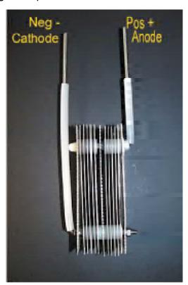
Next, leaving all but the starting nuts loose, the two halves can now be assembled to make the entire unit. I have to stress this issue about tubings that need to end against a nut & washers that slip over tubing need to do just that, because they can & will move until put in their correct order upon tighting the final nuts. Cut plastic tubings to leave enough thread to allow a nut & washer, plus a little at each of the ends.
