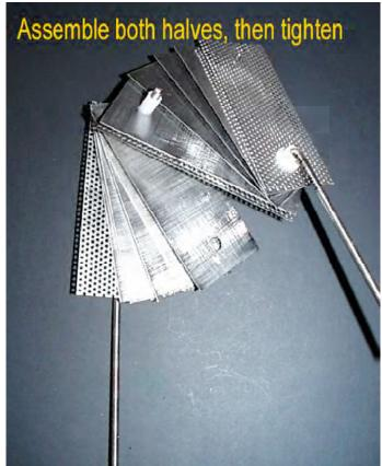
This detail shows Pos - Anode assembly, note that Pos plate is secured w/ a thin nut on either side of the + plate, on the Pos rod. Workout the length of the short pieces of tubing between the center + plate to insulate the neutral & Neg - end plates from the Pos + rod.
