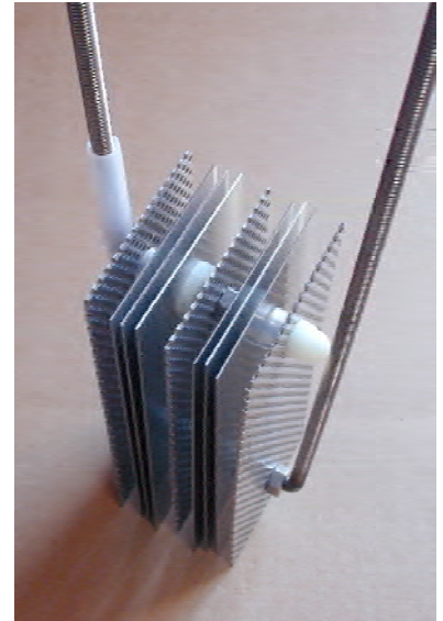
Photo of a 9 plate assembly, for 11 plates just add 2 more solid (neutral) plates.
